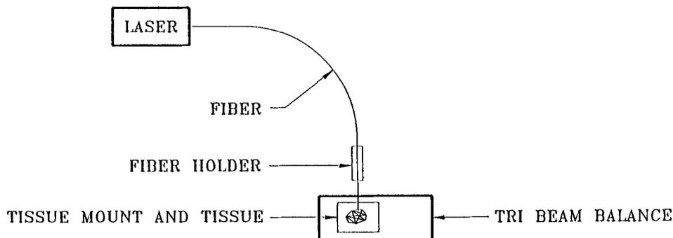
Fig.1. Fixture setup demonstrating penetration rate.
