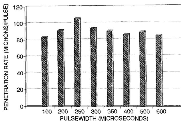
Fig. 2. Histogram of penetration rates vs. different pulse widths (0.5 J/pulse @ 5 Hz).
